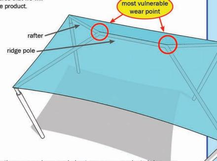
Over the years we have carried out numerous repairs to bring worn shadecloth covers back into servicability. Whilst the Shadeport is undoubtedly one of the most durable and low maintenance shade products available, when carrying out repairs the most common wear point is where the rafters meet the ridge pole. Because the Shadeport fabric is tensioned over the steel frame, the fabric is in contact with the framework and thus wear can occur under wind loading over a period of time.
